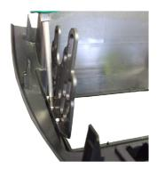
Using screws supplied, screw the head unit to the brackets on both sides.
