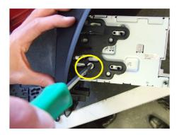
12. Screw the facia in place (reverse of step 2) Re-attach the button removed in step 1.
