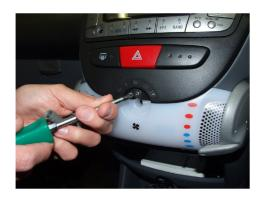
Lift the bottom of the panel upwards and pull the panel out.
