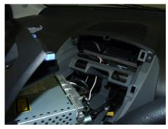
5. Unscrew the centre screw from the plastic housing at the rear of the aperture (circled).
