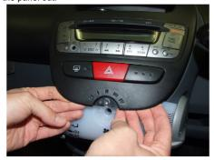
4. Disconnect the three buttons from the rear of the panel. Remove panel and put to one side.
