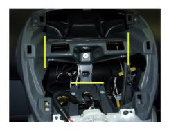
3. Disconnect the connectors from the back of the head unit.
