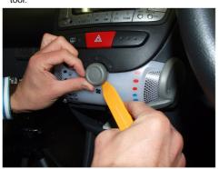
Remove the screw which is behind the fan control button.
