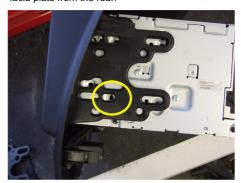
11. Re-connect the buttons (reverse of step 4). Connect the wiring harness and the antenna from the car to the aftermarket head unit. Insert the aftermarket head unit and facia into the dash. The facia clips in as the original facia panel does.
